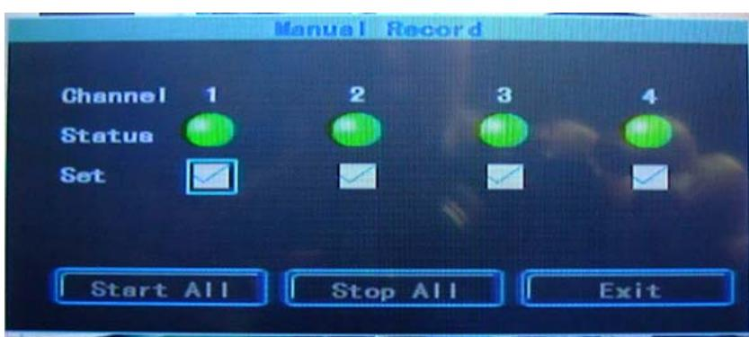
Select the cameras you want to record and start recording with START ALL. It is necessary that the user has the authority to start recording and an SD card is inserted into the slot.
