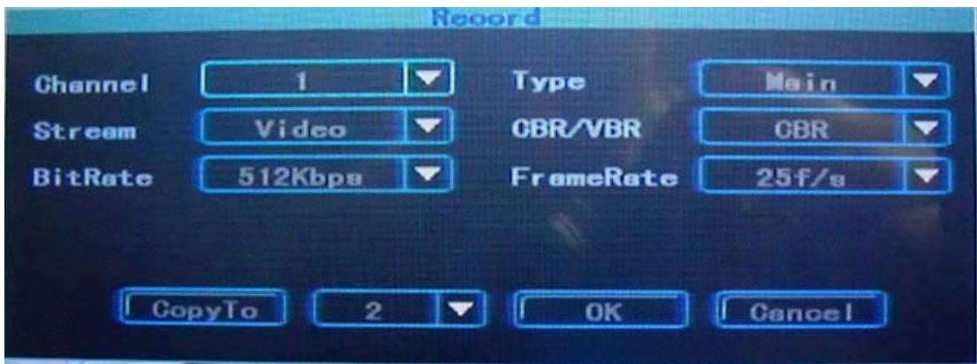
This section allows you to set the video parameters of the 4 channels
