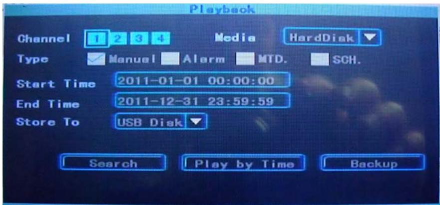
You can choose the channels to be reviewed and the type of recording. In the spaces START TIME and END TIME to set the time period over which to search. In MEDIA space select SD card. You can also choose which types of recording search: MANUAL: Recording started with manual control ALARM: Off
