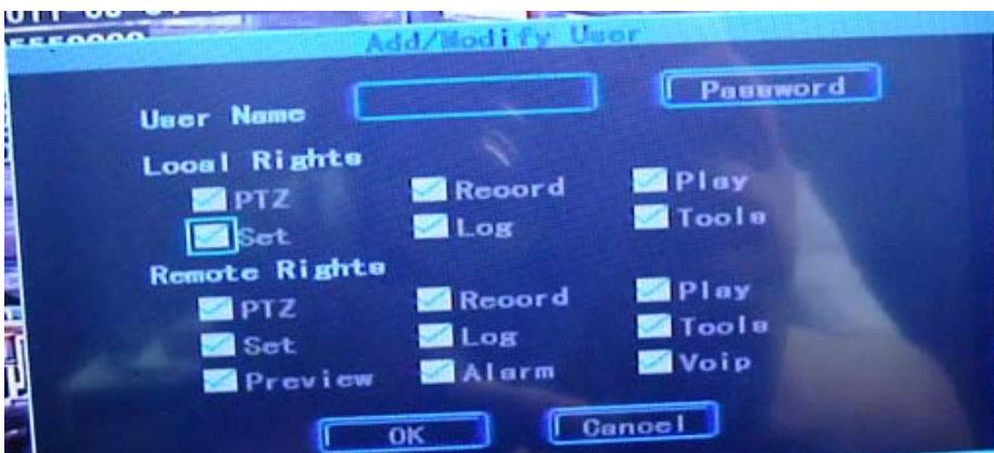
And 'possible to enter a user name with characters and numbers (change modes with the fn key) and the access password. Then they define the authorized access. This DVR, in consideration of its use, does not allow remote connection for which you can only define LOCAL RIGHTS (Local Rights). RECORD (check register), PLAY (watch recordings), the SET (programming), LOG (event memory), TOOLS (voice of programming TOOLS).
