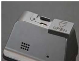
It can use micro SD card with a capacity of 4 to 128 GB CLASS 10 or higher.
