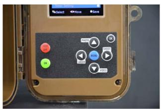
First, you notice that the device has two power buttons: TEST / OFF and ON
