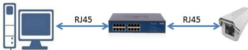
As soon as the mains and power supply are connected, check that the switch port LEDs start flashing. This means that the camera is working and you can continue to configure the IP address.
