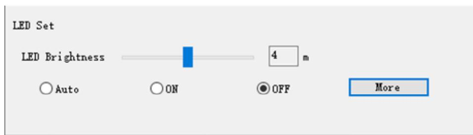
AUTO - The illuminator switches on automatically based on the rear light sensor OFF - The illuminator switches on based on the back light sensor only within the time bands set in the configuration menu, PERIPHERAL / LED section. Outside the defined time bands, the illuminator remains off.
