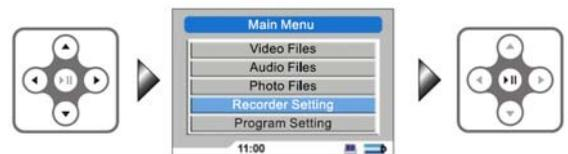
Select RECORDER SETTING and press ENTER. You are offered three options: Audio Line, Line Video and Motion Detect.
