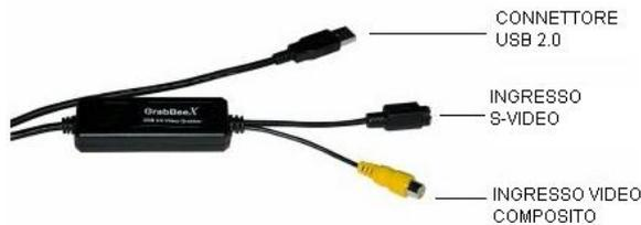
Connect the USB connector to a USB 2.0 port on your PC. Through this port, as well as communicate with the PC, the device will receive the power.
