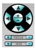
**PTZ controls.** If the selected camera is a dome camera connected to the DVR you can control it remotely. The control panel includes Tilt Up / Down, Pan Left / Right, Zoom In / Out, Focus Near, Focus Far, Iris - (darker), Iris + (brighter).
