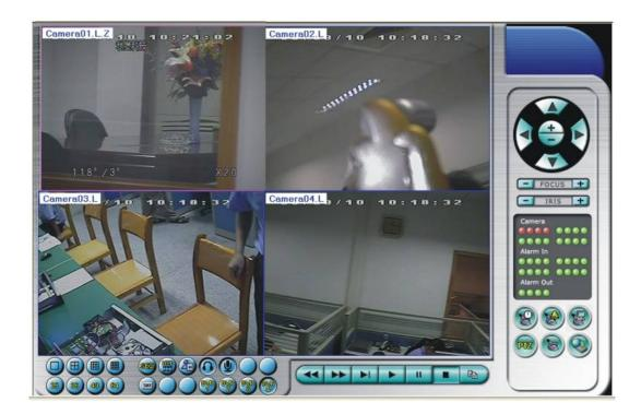
The display window can be divided into several boxes containing 1 or 4 cameras. The cameras whose name is followed by the letter L are viewing LIVE, those followed by the letter P in the playback mode. The cameras As highlighted in white are detecting intrusion (Motion).
