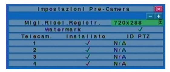
Up to 4 cameras can be connected to the system. The pre-camera settings allow the administrator to define some fundamental attributes for all the installed cameras.
