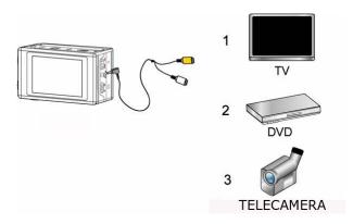
In addition to CCTV cameras, you can connect other video sources such as DVD players, VCRs and TV to record programs. Depending on the connections of the device to be connected you may be required
