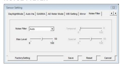
It is possible to set the digital reduction of video noise automatically (with max adjustable threshold) or manually (with adjustment of time and space thresholds). The SPACIAL setting reduces the noise in the single frame, while the TEMPORAL setting defines the interval of the frames.
