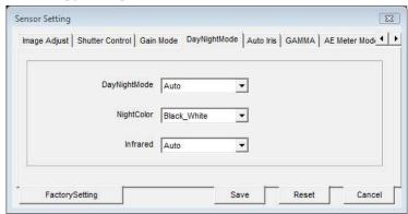
In this tab you can set the behavior of the day / night function. The window may include more or less options depending on the camera model in question. DAY / NIGHT MODE - Set to AUTO it enables automatic switching to night mode when darkness falls. Set to Day or Night mode it always forces a COLOR (DAY) or B / W (NIGHT) mode regardless of the ambient brightness. In some models it is also possible to define the thresholds of the day / night changeover or decide to do it on an hourly basis.
