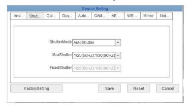
Adjusts the speed of the electronic iris to be defined according to the ambient brightness. A slow diaphragm is very bright with little light but is likely to cause bleaching in case of strong daylight. On the contrary, a fast shutter will be excellent in a bright environment but could give underexposed images in low light.
