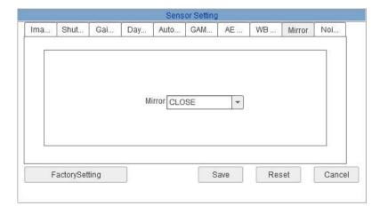
It is possible to invert the image to adapt the vision to the position of the camera.
