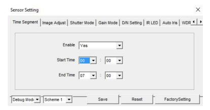
In the window it is possible to set when to activate the selected configuration scheme (1,2,3,4) with start and end time.
