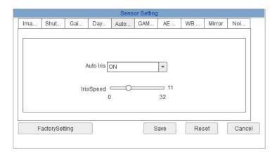
If the camera uses an auto iris lens it is possible to set the actuation speed. In the case of a fixed lens, leave the setting OFF. In AUTOIRIS OFF mode the priority of the brightness adjustment is given to the electronic shutter. IRIS SPEED indicates the reaction speed of the lens. Reduce the speed if the lens were to open and close continuously giving a flash effect in certain light conditions.
