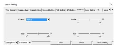
In some models it is possible to adjust the power of the LED lighting to avoid excessive bleaching in close-up shots. In this example (Speed Dome 3MP) there are 3 adjustment levels for close-up, medium and long distance shooting based on the zoom level set.
