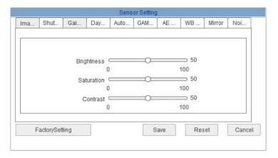
Allows you to adjust Brightness, Saturation and Contrast in the image. Some models also offer additional options.
