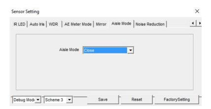
In some models it is possible to enable the corridor mode which allows you to change the resolution of the camera using the greater value on the vertical side instead of the horizontal one. This type of shot can be effective when shooting a long narrow area such as a corridor.
