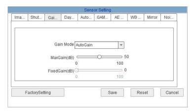
Allows you to adjust the sensor gain. It is possible to set an automatic value (with adjustable maximum threshold) or a fixed value.
