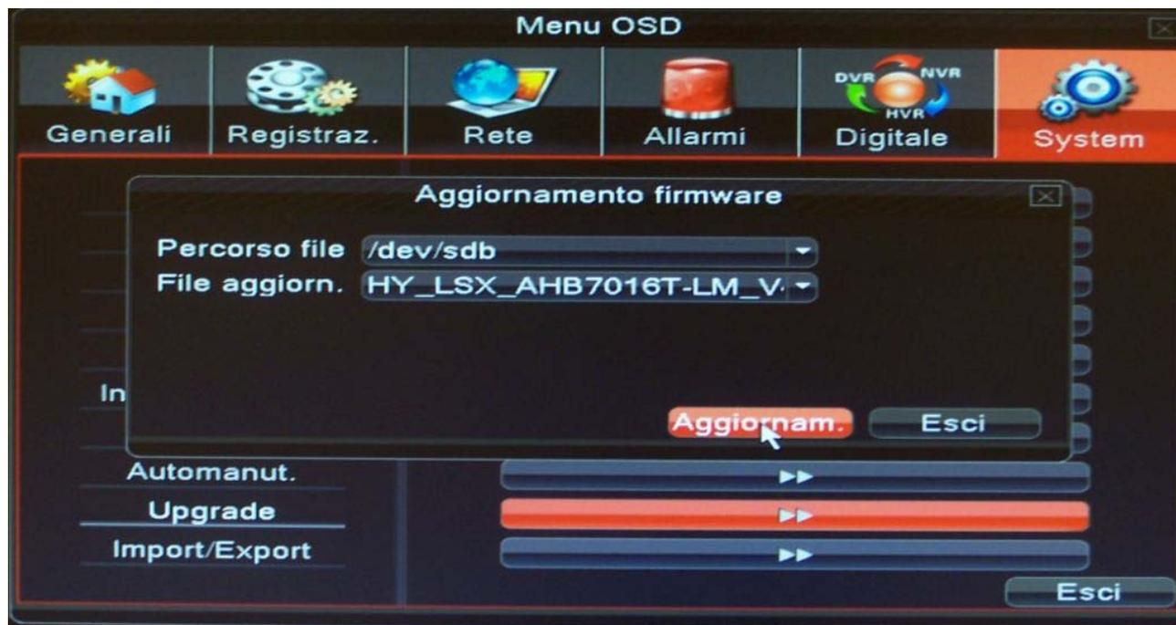
This section is used to update the internal software of the DVR. To perform this operation you need to get from our technical service for the upgrade file and copy it to a USB key to be inserted into the DVR.
