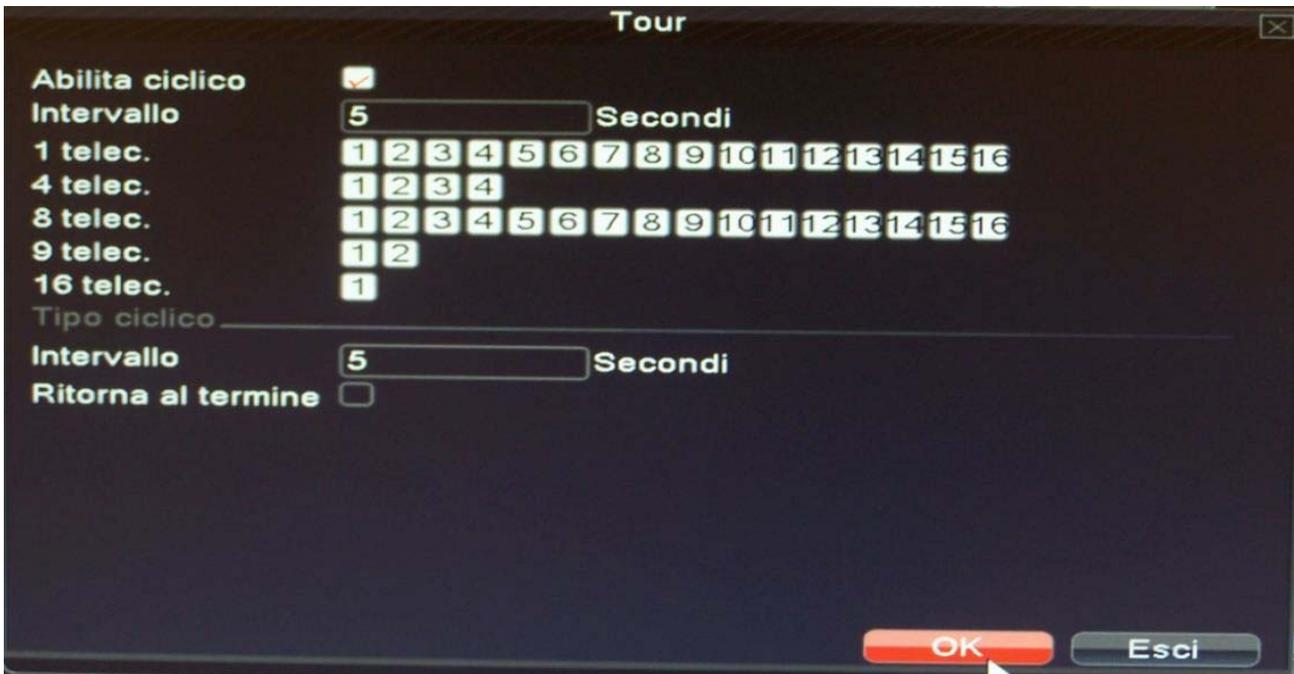
First you need to enable the cyclic and define that interval of time will pass between one screen and the next (INTERVAL: 5 to 120 sec.).
