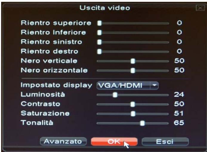
In the upper section adjusts the size of the screen and in the bottom section of the rendered image.
