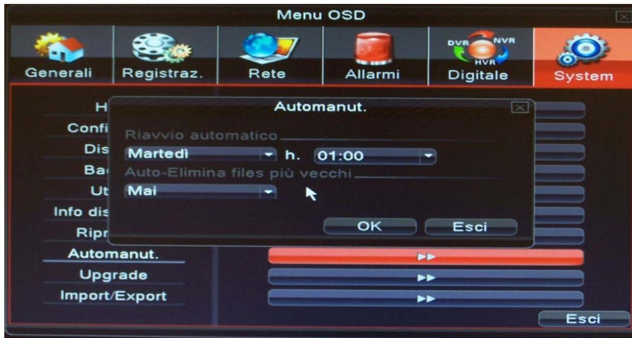
This section serves to program two automatic functions that the DVR will automatically perform a regular basis.
