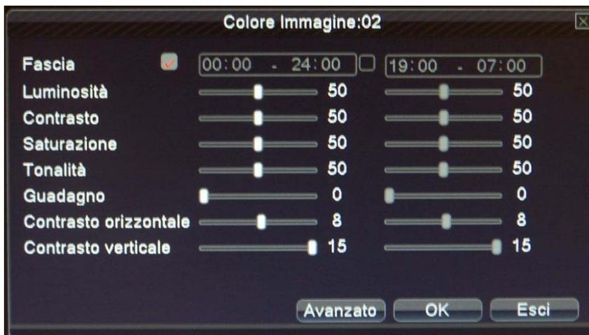
And 'possible to adjust the image parameters and set if desired two daily time slots with different settings (eg. Day / night)
