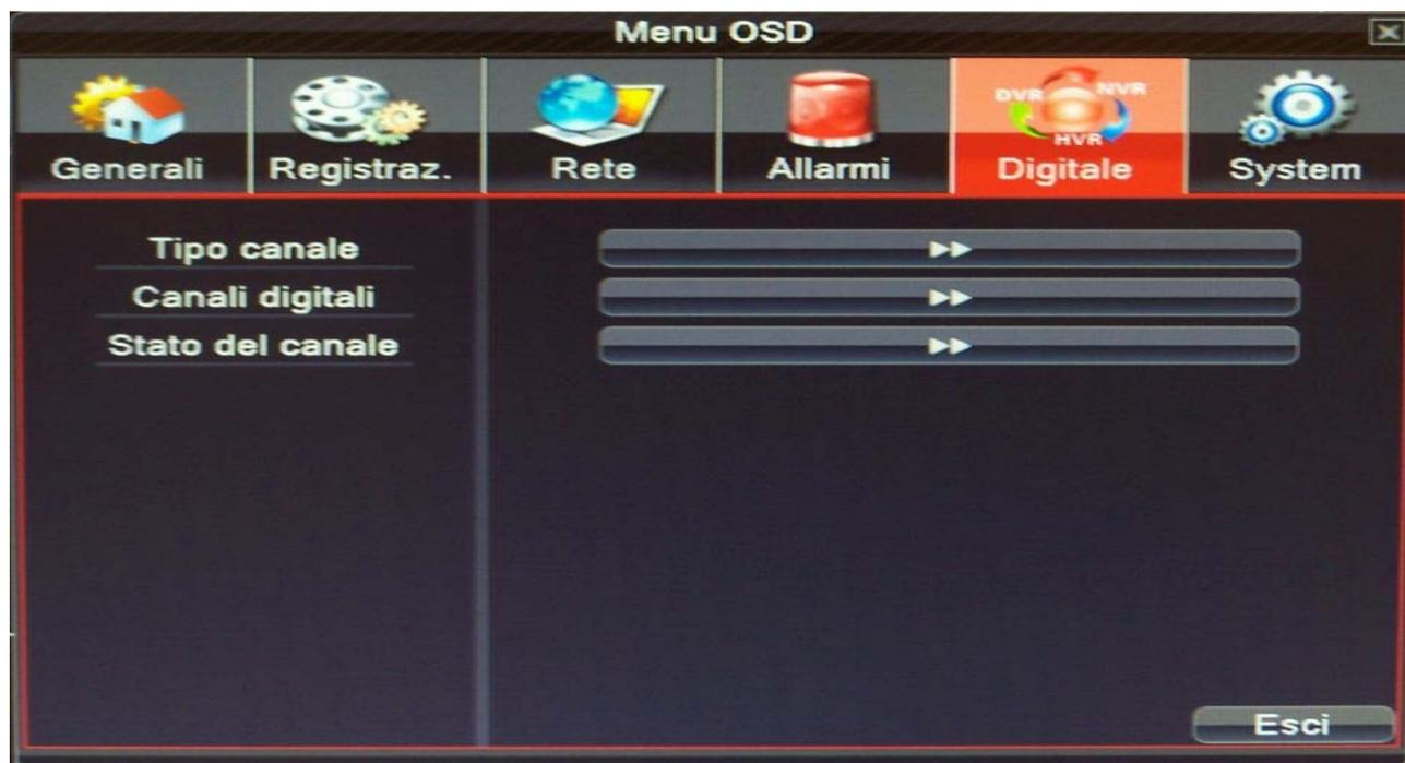
Clicking DIGITAL CHANNELS You can connect the IP cameras on the network to the DVR / NVR if you have not already done so with the configuration wizard seen above.
