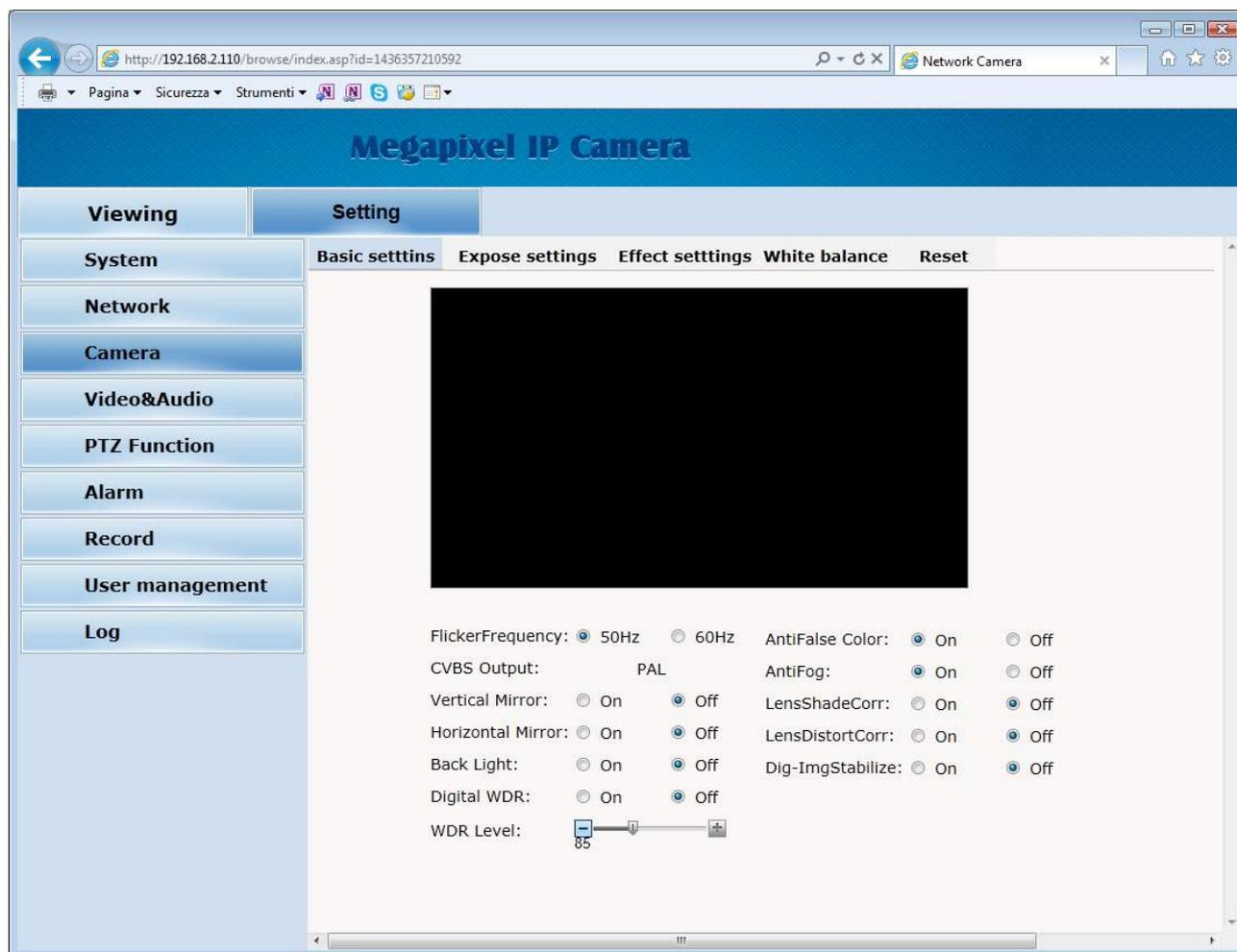
The CAMERA page, with its various tables includes configuration parameters of the module camera with the usual image adjustment items.
