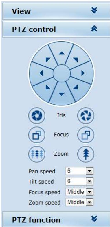
In this window you control the camera movements. The movements are controlled with the mouse buttons while the IRIS, FOCUS and ZOOM intervene on IRIS, FOCUS and ZOOM. In this parameter, the zoom is always controlled and IRIS FOCUS and can not be active if the camera settings provide automatic capabilities. At the bottom it is possible to adjust PAN SPEED (horizontal movement speed), TILT SPEED (vertical movement speed), FOCUS SPEED (firing rate) and ZOOM SPEED (zoom speed).
