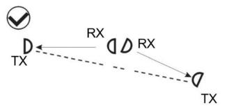
The barrier can be operated even if the transmitter and receiver are not on the same line, if it falls within the following maximum horizontal and vertical tolerances.
