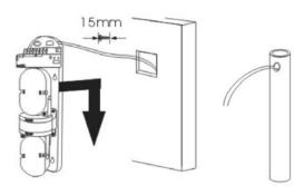
If you want to install the barrier on a pole includes two collar plates. Here it is shown a classic mounting back to back.
