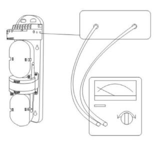
When the barrier is properly aligned on the tester you will need a voltage of at least 1.2V. Act on guidance mechanisms to achieve the highest possible value.
