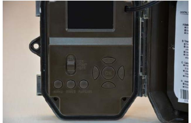
First, to start the device and configure its options, you must move the main switch in the TEST position, in this way the equipment is started.
