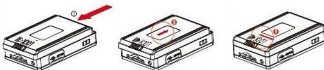
**Inserting SD card** - The commissioning of the device, the first thing to do is to install the SD card. E comes with the product an SD card 4GB which allows over 1.5 hours of HD recording. Aside you can also buy memory card with different storage capacity as our DK-MSD32G (32 GB). E, however, use any SD-card without Brand limits or abilities and also microSD card using the adapter provided.
