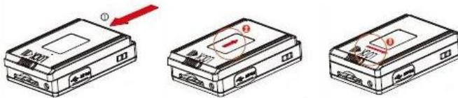
**Inserting SD card** - The commissioning of the device, the first thing to do is to install the SD card. E 'comes with the product an SD card 4GB which allows about 6 hours of recording. Aside you can also buy memory card with different storage capacity as our DK-MSD32G (32 GB). E ', however, use any SD-card without Brand limits or abilities and also microSD card using the adapter provided.
