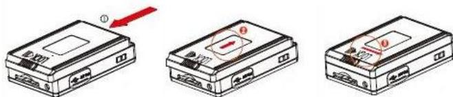
**Inserting SD card** - Before turning on the DVR, the first thing to do is to install the SD card. Without SD card DVR does not start.
