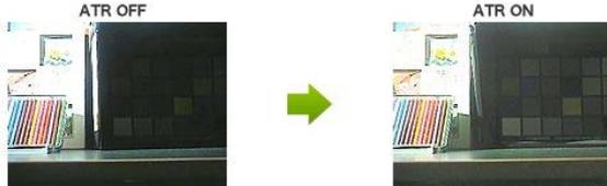
By activating this function (ON), it is possible to shoot in backlight of a dark subject on bright background with the maximum result. Compared to the above mentioned BLC This function allows you to make the dark subject and simultaneously visible the bright background which typically ends in BLC overexposed. Pressing ENTER ON you can change two parameters for shooting: LUMINANCE (brightness) and CONTRAST (contrast).
