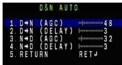
By choosing the AUTO option it is possible to set the thresholds (AGC) for day / night (DN) and night / day (ND) passage and a possible delay (DELAY). The delay is used to avoid unwanted passages due to rapid changes in brightness.
