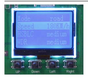
**MODE** - The first menu item allows you to auto-configure all subsequent options quickly simply by selecting the type of camera use. Select PARKING if you are using the camera in an area where vehicles are moving slowly, such as in a parking lot or service area. Select ROAD if you want to monitor a road with fast moving vehicles.
