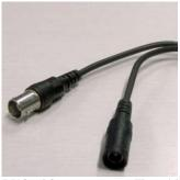
**BNC video output** - The video cable is connected to the bayonet female BNC connector and then leads to an AHD DVR.
