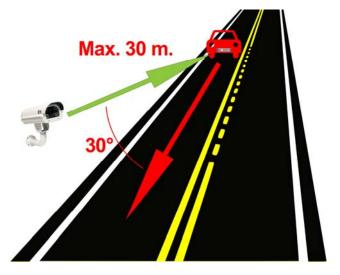
You can frame from 1 to 3 lanes, depending on the lens setting. See in this example an optimal 3-lane shot
