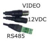
**BNC video output** - At the BNC female bayonet connecting the video cable that leads then to monitor or management devices typically using RG59 coaxial cable and BNC connector. The RE-BCC8HD cameras are cameras that can work with both conventional analog DVR or DVR
