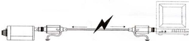
**RE-PR2 - Video Input protection of RJ45 and twisted pair CAT5 cable.** The security module RE-PR2 has the same security features of the RE-PR1 model, but it is developed to protect video transmission over twisted pair cables is performed using the appropriate balun converters. E' can use the RE-PR2 form both with passive balun converters RE-BNCRJ1 that active.
