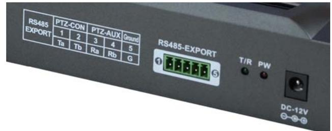
The PTZ AUX terminals are available for connecting a second control panel (Slave). The GND terminal is available to connect to ground the shield of the RS485 cable if necessary.
